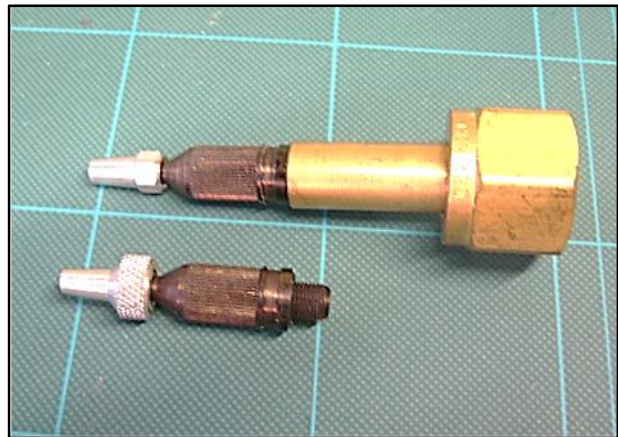
Brown CO 2 fillers from Lindsey Smith's estate. Top, 2mm, with brass adaptor. Bottom, 1.6mm.
