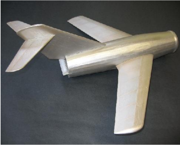
Ducted fan 15" wingspan MiG 15 for Telco Turbotank 3000. The repair to the damage caused by the bursting motor tank can just be seen on the top right of the fuselage. The model was never finished as I could not get it to fly consistently
