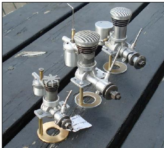
Ouragan 0.9 and 3.3cc diesels with eccentric bearing compression adjustment.
