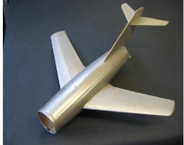
Ducted fan 15" wingspan MiG 15 for Telco Turbotank 3000. The repair to the damage caused by the bursting motor tank can just be seen on the top right of the fuselage. The model was never finished as I could not get it to fly consistently
