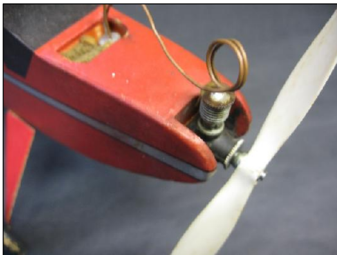
Early Telco motor with eccentric bearing speed adjustment and Williams Bros prop, fitted to all sheet 'Moonco'.
