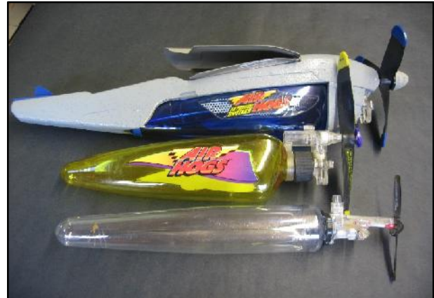
Various Air Hogs units, Blue Sky bottom. The top two larger units appear to have similar motors and similar sized tanks.
