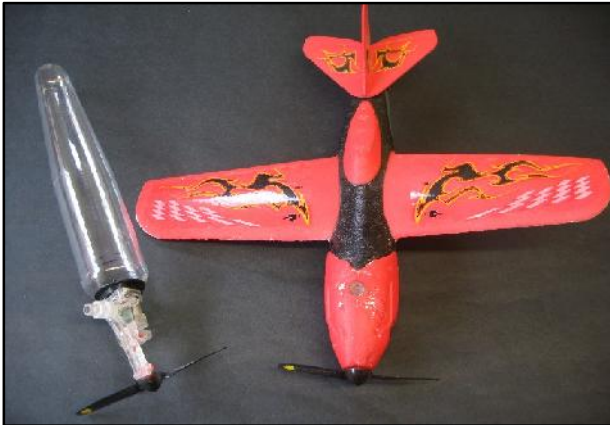
Air Hogs Blue Sky foam plastic RTF, of 12" span, with separate power unit on left.
