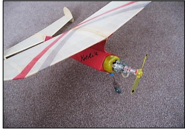
Lindsey Smith's 24" wingspan Hot Air with Air Hogs Blue Sky compressed air power unit.
