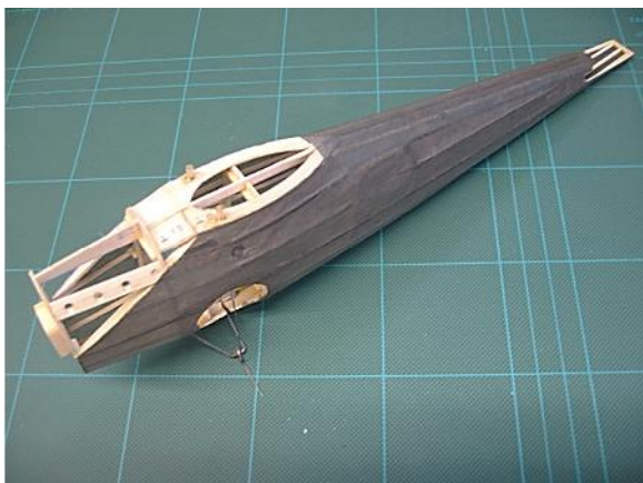
Covered fuselage prior to shrinking the tissue
