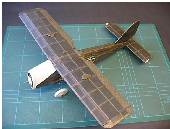
Components covered, tissue shrunk and thin dope oil applied. The nose is covered with doped copier paper.
