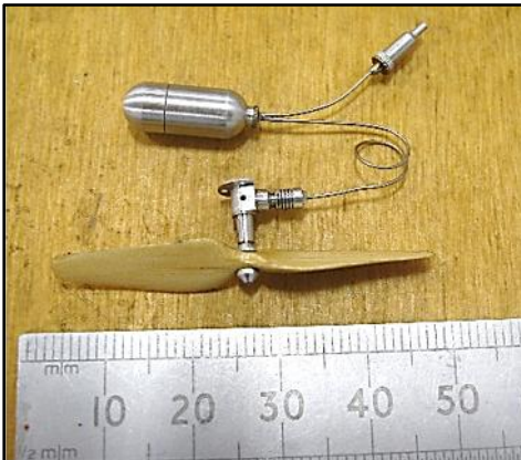
GM07 motor – all of 0.7 mm 3 capacity!
