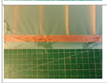
I normally start at one point at one end of the wing, then one point at the other end of the wing, then the four corners, then multiple points along all the edges...
