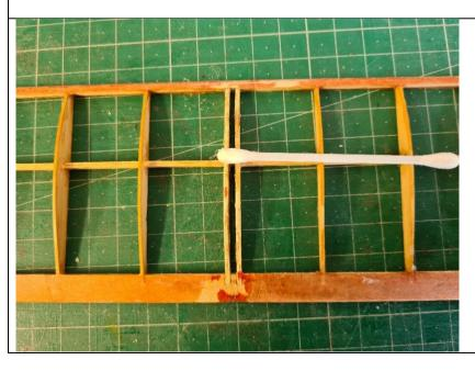
Same for the tailplane but for a different reason. The top covering I've done as one piece and when the slot for the fin is cut in the covering all the tension will be on the adhesion to the centre ribs. This can be mitigated by a bead of glue to the fin when the fin is replaced.
