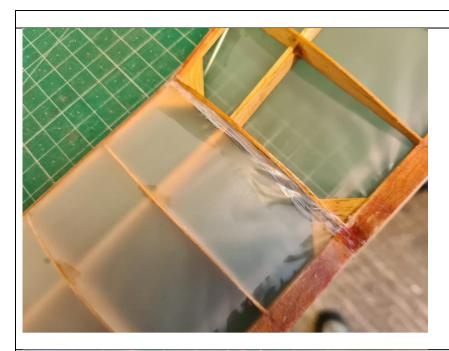
The top surface is dealt with in a similar way but has to be done one wing at a time because of the dihedral. At the centre I've ironed down a few millimetres down the side of the centre rib.
