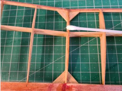
Doculam has an adhesive layer but in this case, there isn't much surface area to adhere to. To assist in preventing the doculam pulling away from the centre rib as it shrinks I've applied a small amount of cover grip to the top of this rib.
