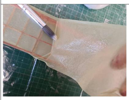
Getting more delicate here, the tissue will expand so lift carefully and lay back, using the brush as you go to smooth it out. This is where wet strength is necessary. Note the relative copious amounts of Ezedope. Too much is much better than too little. Brush out the air bubbles as you go. It may be necessary to lift the tissue several times, both from left & right and up & down.
