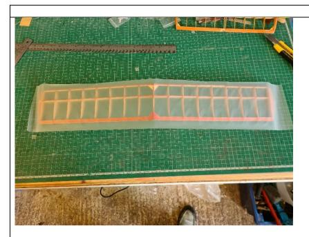
For the wing I've cut a piece of doculam somewhat bigger than the overall size. And starting with the lower surface.
