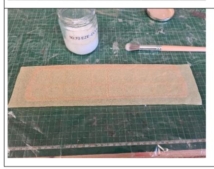
Starting on the underside, cut a piece of tissue around 10 – 15mm oversize. The tissue must have good wet strength, I'm using Deluxe Materials Eze-tissue.
