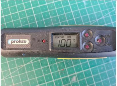
Starting with the iron set as low as possible, 100 deg C in this case, start tacking down.
