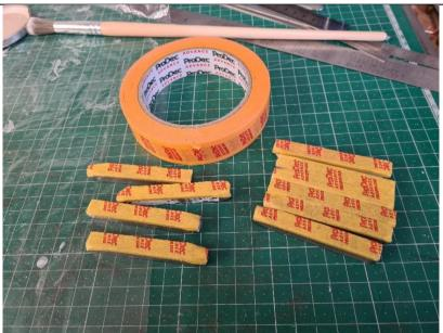
For me, my building technique has evolved to use weights & a nice flat surface rather than pins, but no matter, work as you see fit. I use letter stamps as weights & spacers. To stop the workpiece sticking to them I apply some masking tape to one side. Spacers will be needed to allow airflow under the workpiece, these can be wood packing pieces. Use suitable tape to stop unwanted adhesion.
