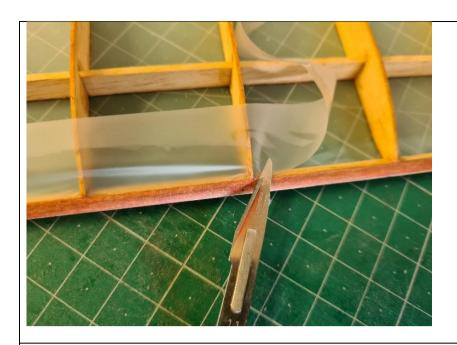
Trim off excess at the leading & trailing edges. I leave a few millimetres to wrap round the leading edge & none at the trailing edge.
