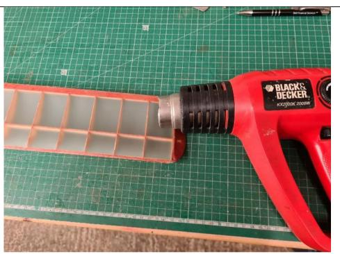
The best bit! Using the lowest temperature that will work, shrink the doculam.
