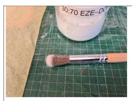
And the messy bit! A bit of preparation is needed before starting. Mix up sufficient Eze-dope beforehand. Notice the polythene sheet over the building board. And the large very soft brush.
