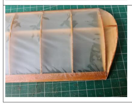
Tacking down the second piece. At the wing tip I've cut a few millimetres over size, made a few cuts, and ironed down it down over the edge.
