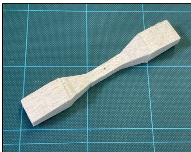
Fig 10. Sawn prop blank the key to successful propeller carving
