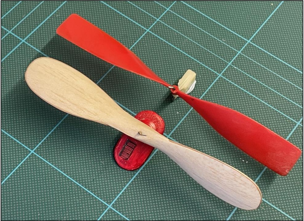
Fig. 11. Finished Swallow prop in comparison with the Sleek Streek plastic prop.
