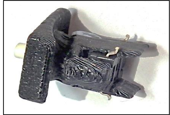
Illustration 5: Assembled start button note curve to fit tubular fuselage
