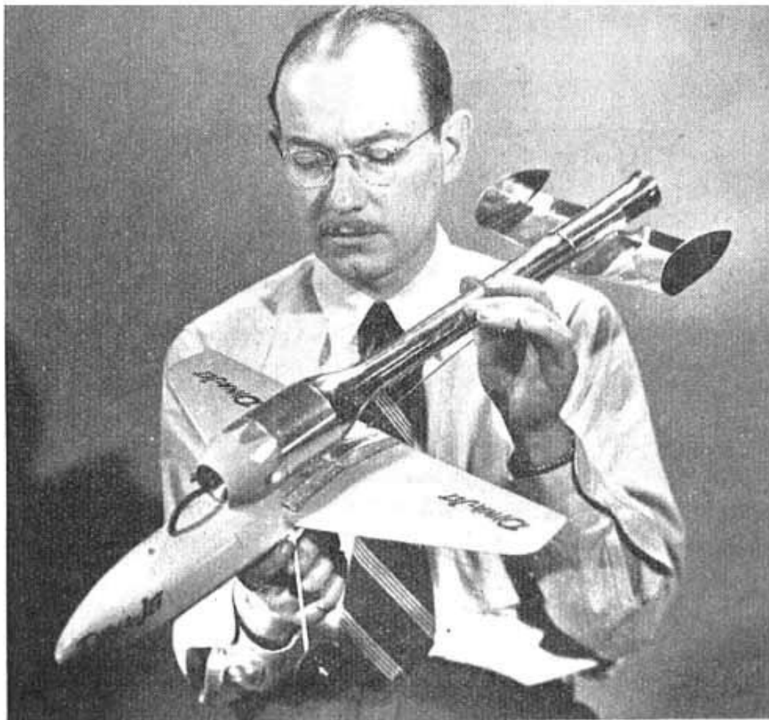
The latest Dynajet control-line racing model with solid balsa wings and metal tailplane. Note that in this model the tail fins are made from sheet metal and the unit is clipped on to the jet engine units tailpiece.
