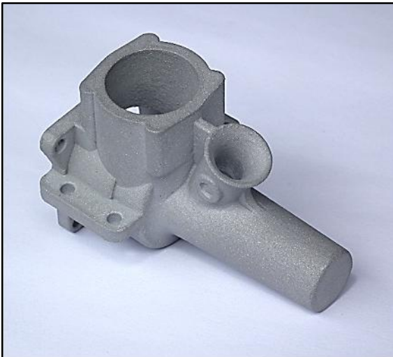
Illustration 1: Sugden Special crankcase 3D printed in aluminium
