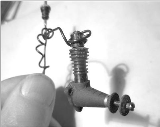
BJ .005. The pipe feed to the top of the cylinder has clearly been modified
