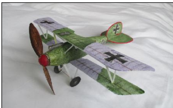
Wallpaper foam Albatross DV. The fuselage has been made by binding the foam around a wooden form
