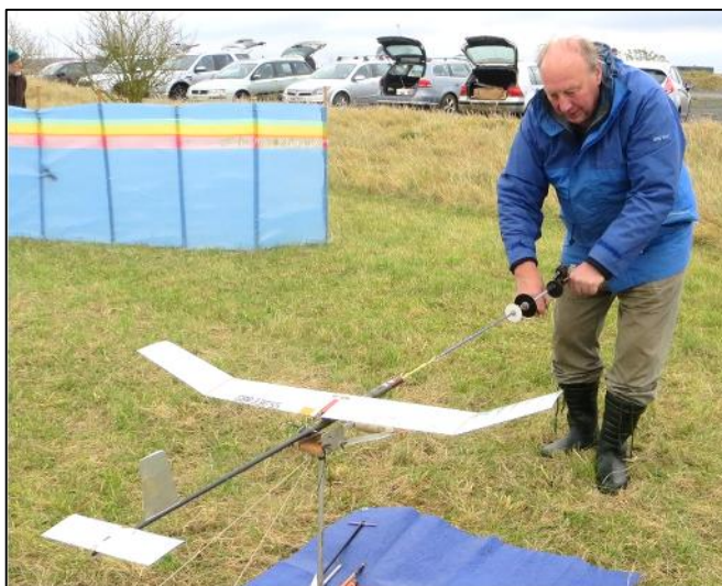
Phil winds his motors outside the model using a half tube for loading, Steve winds conventionally, breaking his motors in the blast tube.
