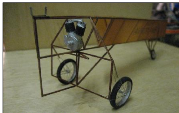
Fuselage for a Pistachio scale Roe Triplane I 'Bulls Eye'
