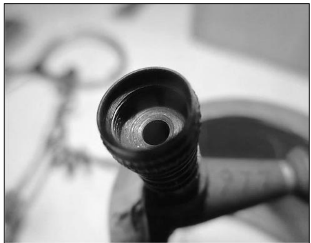
Top of cylinder with cap removed showing the hole where the spigot on piston comes through to lift valve from seat.
