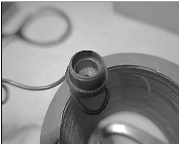
Cylinder cap showing large recess to accommodate valve
