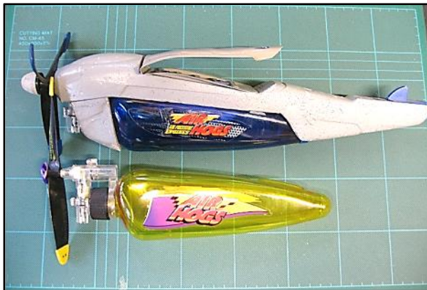
Air Hogs Sky Shark fuselage and motors.
