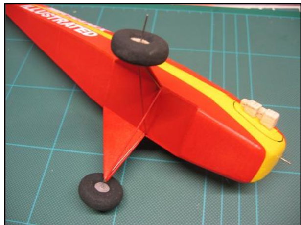
The wheels are mounted on u/c wires not attached to the fairing to give flexibility. The edge of the 'hole' for the engine is marked out.
