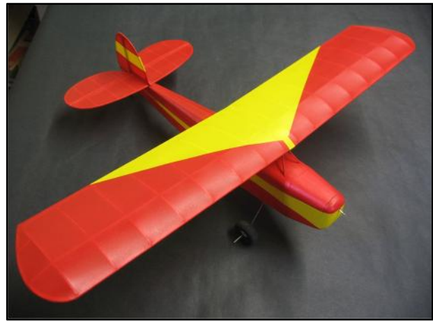
Covering airbrushed with Tamiya acrylic paint, before the application of registration and other letters.
