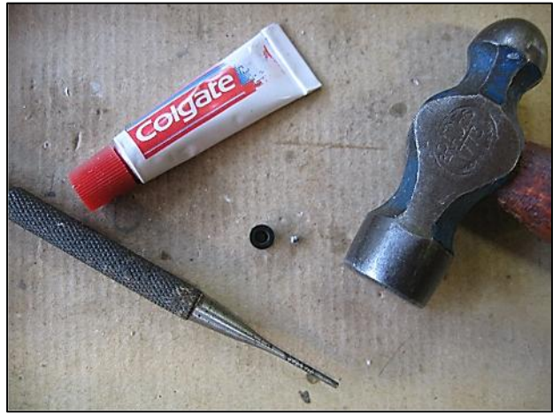
Equipment required to improve valve seat sealing shown with Telco valve seat and 3/32" dia ball.
