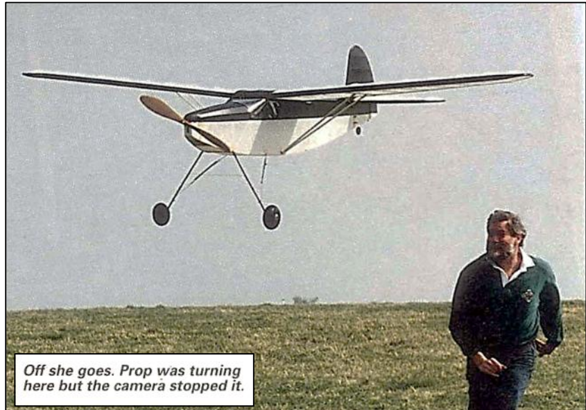
The tailplane is secured by the fin, an arrangement that did not allow sufficient adjustment. Easy to alter but not on the field.
