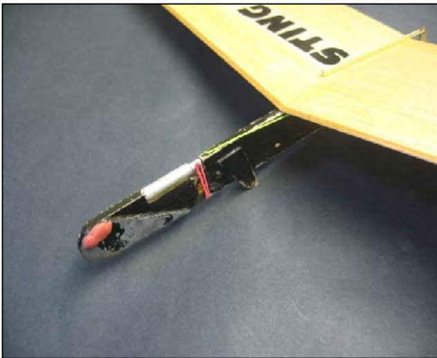
'Cool tube' installation in Len Surtees' Sting 18 CLG. The inner tube is rotated by the red elastic band, eventually releasing the pivoted rear boom.
