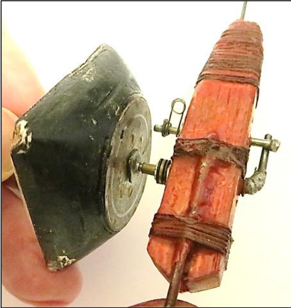
Fig 1: shows the assembly in the power drive position with the prop shaft drive arm holding the spring loaded pin away from the noseblock faceplate
