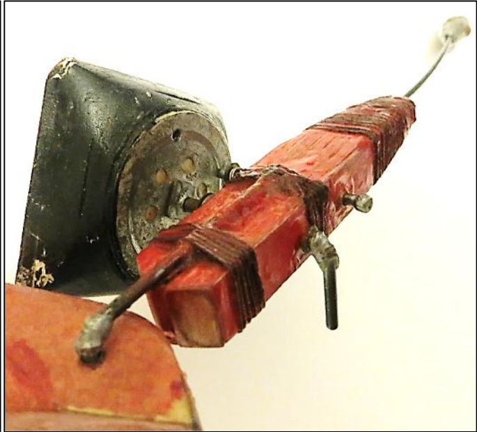
Fig 2: shows the assembly shortly after power is exhausted. The prop shaft drive arm has disengaged from the spring loaded pin which is now rubbing on the noseblock faceplate as the prop rotates until the pin drops into the stop hole
