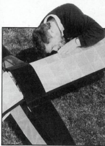
Model assembles easily; break in the two-piece fuselage can just be seen behind wing where it is held by a small rubber band at each corner.
