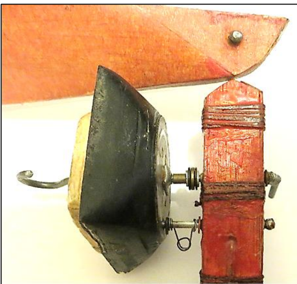
Fig 3: showing spring loaded pin fully engaged in hole in noseblock faceplate, locking the prop assembly in the folded position
