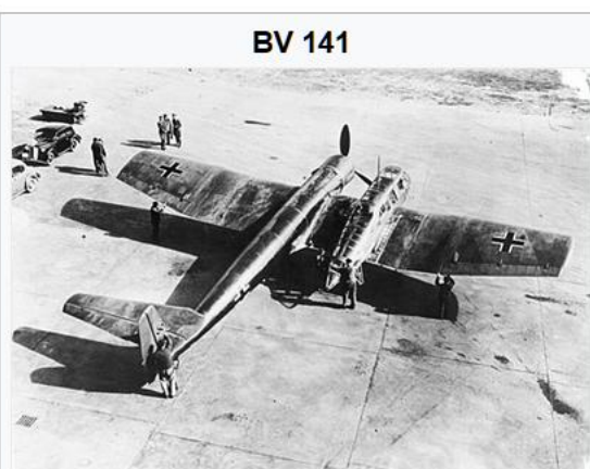
BV 141B featuring its asymmetrical gondola and tailplane.
