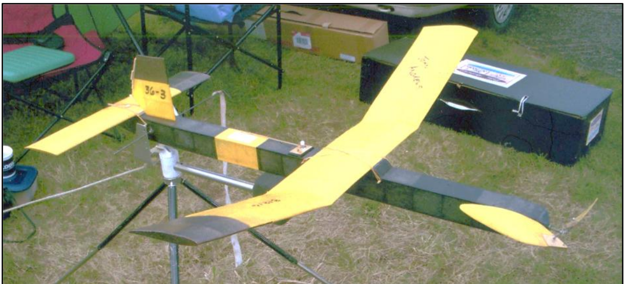
After my re-birth as a Free-Flight rubber flyer, the early version of this model was my first competition flyer. Originally it did not have a wing mount and used a fuse D/T, but after I set fire to it on Warwick racecourse whilst lighting the fuse, the back end was rebuilt with Tomy timer and wing mount added as above. I also increased the wing span at some time.
