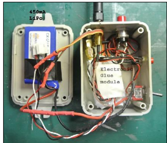
All the Tx components fitted into the Maplin box
