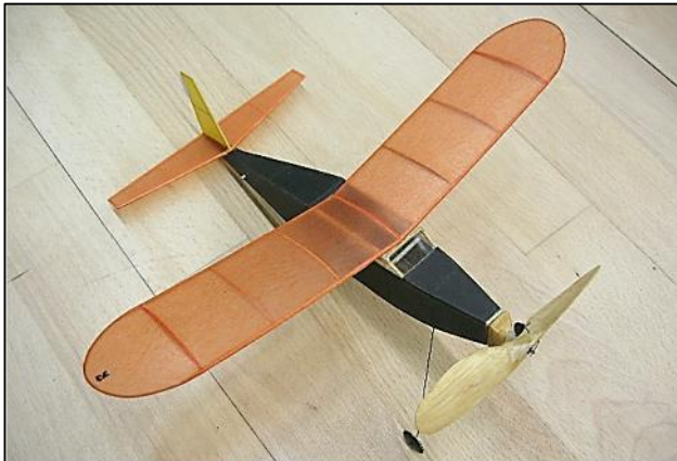
Alan Orthof designed Parlor Fly from 1937 Flying Aces built by Rod Green. 11 in wingspan.
