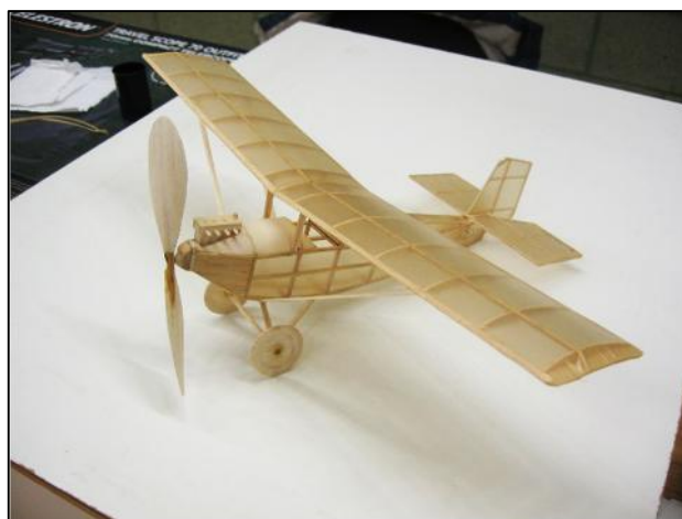
Two more Peanuts: - Bryan Stichbury's 1906 Santos Dumont 14bis and Alisdair Clark's Peck 1928 Pietenpol Air Camper, which is condenser paper covered and weighs less than 10g with rubber.
