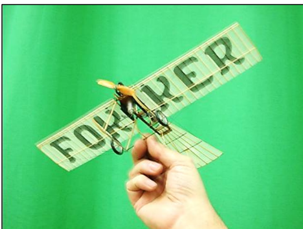
Pete Iliffe's version of Anthony Fokker's Spin (Spider), his first aeroplane from 1910, powered by a Gasparin G10 CO 2 motor
