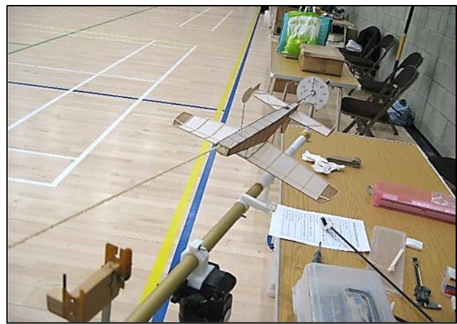
Terry Adams Legal Eagle winding arrangement with torque meter
