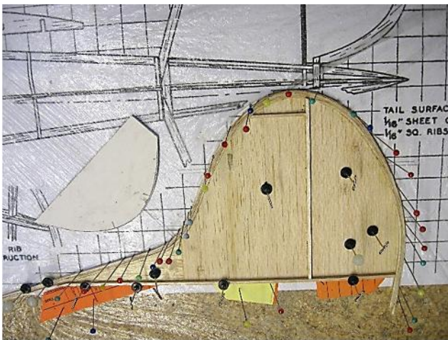
Fin and rudder under construction, the spars are 1/16" x 3/32" deep. The card form was used to help form the reversed curvature in the laminations.
