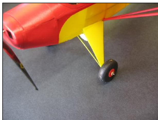
Fig 4. Laminated and turned balsa wheel on KK Piper Super Cruiser
