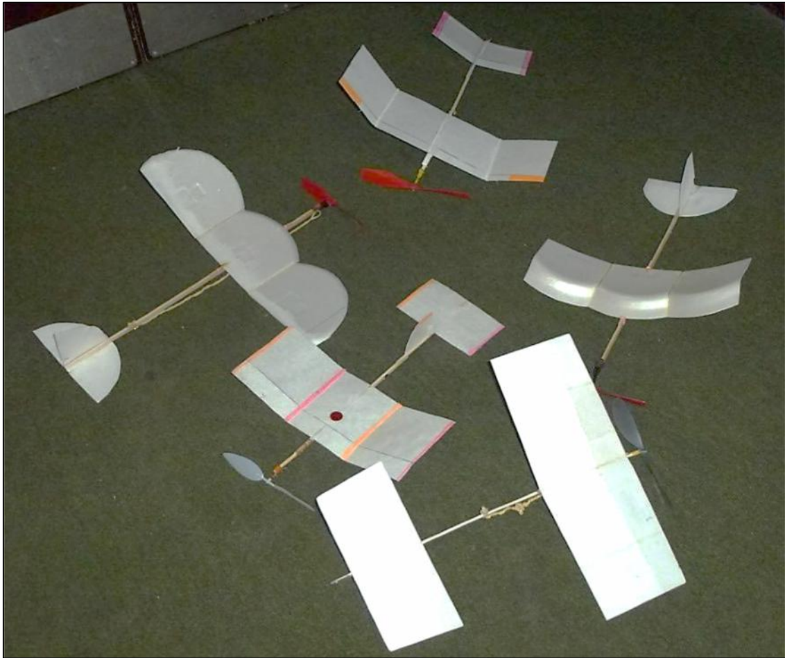
A selection of models made from cut up polystyrene picnic plates All must use a standard commercial prop. They go best without the curry sauce on them.
