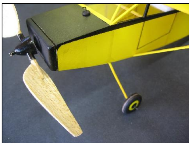
Fig 3. Finished plastic wheel on Cougar. See the tracking mark where it has run on the ground.
