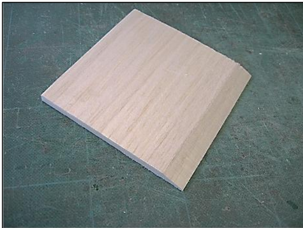
Tapered form on 1/4" sheet used to make cowl blisters
