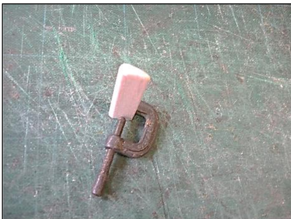
Tear drop section formed and end rounded. The clamp is just holding the piece in position for the photo.
