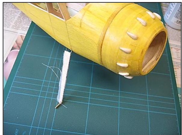
Blisters glued to cowl and attachment of sheet balsa UC fairing.
