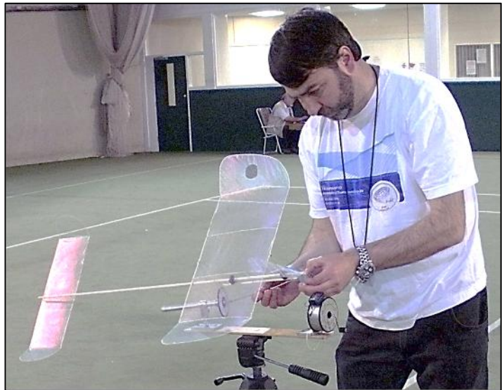
Mark Benns transfers his wound motor from stooge to model out in the flying area to minimise danger period before launch
