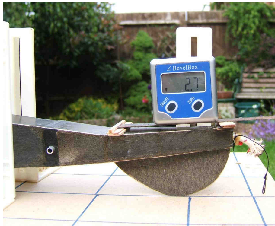
Tailplane mounting = 2.7 deg. underelevated?
