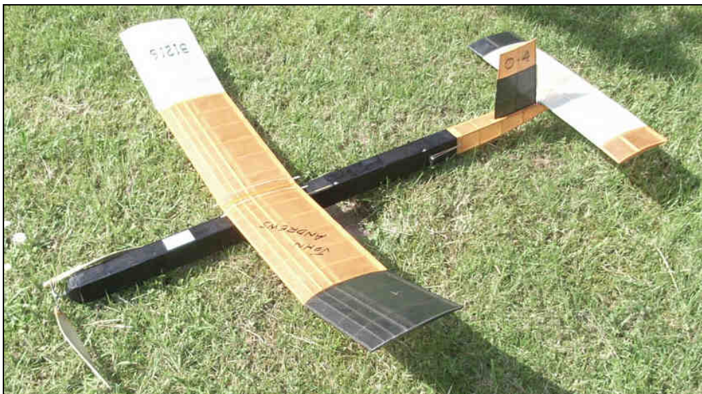
My first new model for a while - O-4 (40" wingspan x 5½" chord, Woodhouse wing section, 80gm airframe)
