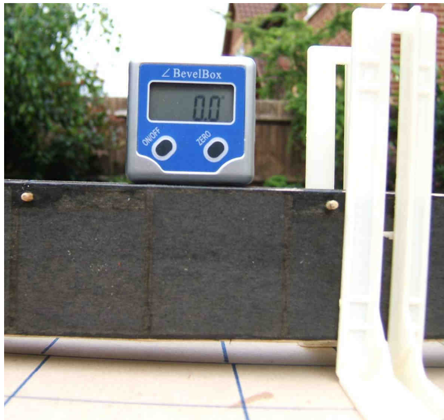
Wing mounting set at 0 deg.
