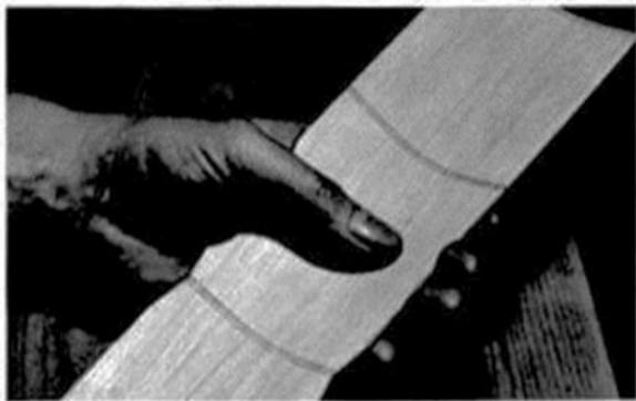
The sheet wing panels must bend easily across grain.
