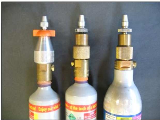
CO 2 motor loading adaptors for SodaStream bottles, from left to right: Telco for 35L, KP Aero for 35L, KP Aero for 60L AICO 2 Jet
