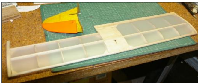
Tailplane and rudder showing locating system carbon rod in rudder and aluminium tube in tailplane with millipede rudder support and elastic band holder.
