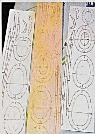
The photocopied formers transferred to 1/16-inch balsa sheet with a hot iron before cutting out (at left). The wing root (above) showing the magnets and locating pegs and holes.
