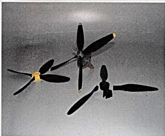
The finished prop assembly and two of the Czech Igra Prop sets (above left) from which the propeller blades were taken. The plug-in landing gear is optional
