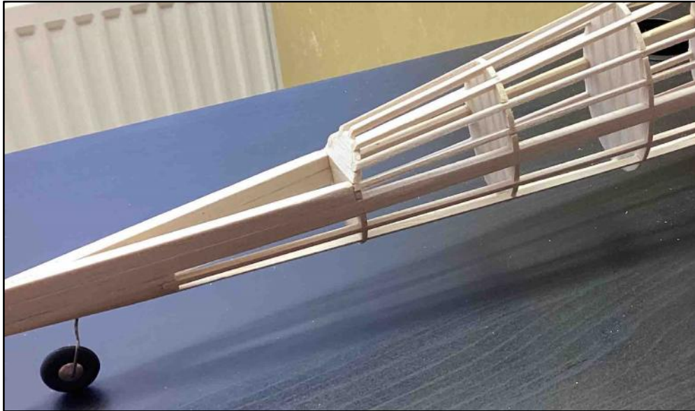
Stringers in place - rear most fuselage former cut & top section tilted forward to facilitate tip-up tail for DT.
