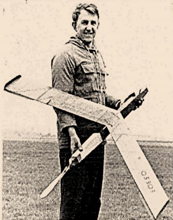
Tail-less winner at Tern Hill was Ken Attiwell with pusher that employs rearward folding prop and side-lifting nose fin for stability.
