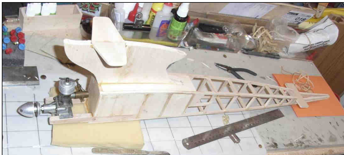
The Jimp fuselage with ED Competition Special power plant now on the building board in the hope of spurring me on to continue construction
