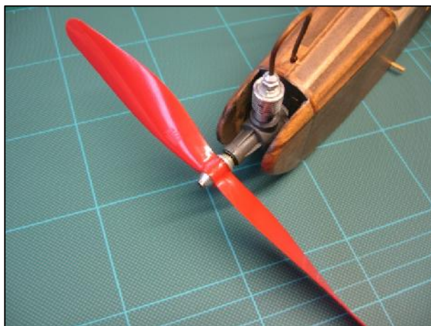
This motor has a grey crankcase, but was retro-fitted with a Gasparin type cylinder assembly.
