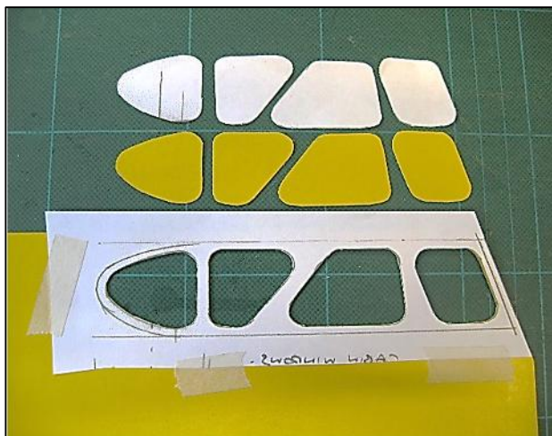
Fig 7. Starboard window frame, with cut-out pieces.
