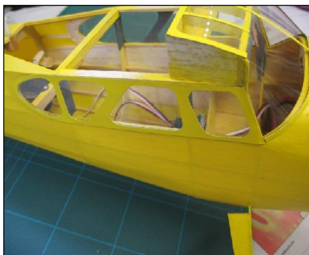
Fig 10. Side window attached to fuselage
