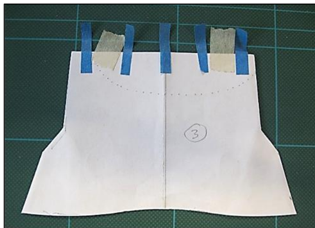
Fig 6. Paper windscreen pattern. The pieces of tape are at the rear.
