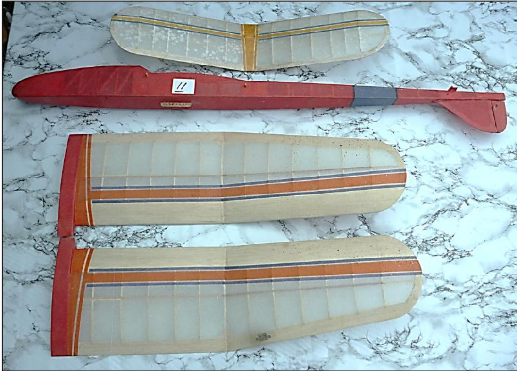
No 11: Wing Span 139cm; Chord 20.5cm; Fuselage length 109cm
