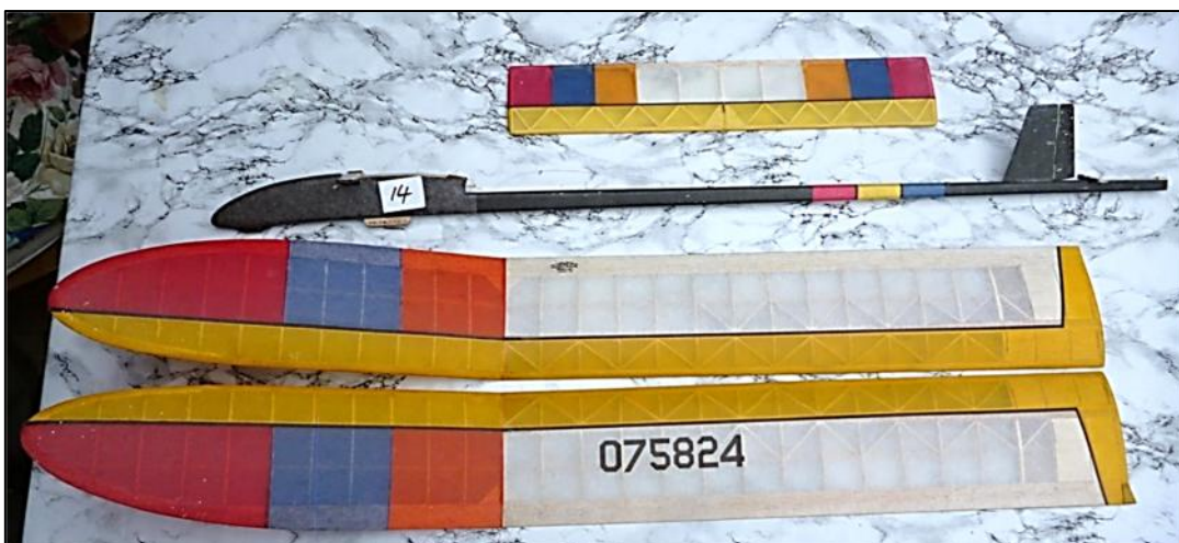
No 14: Wing Span 216cm; Chord 14cm; Fuselage length 110cm
