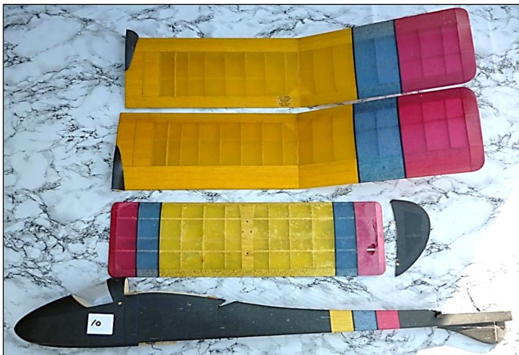
No 10: Wing Span 144cm; Chord 17.5cm; Fuselage length 94cm
