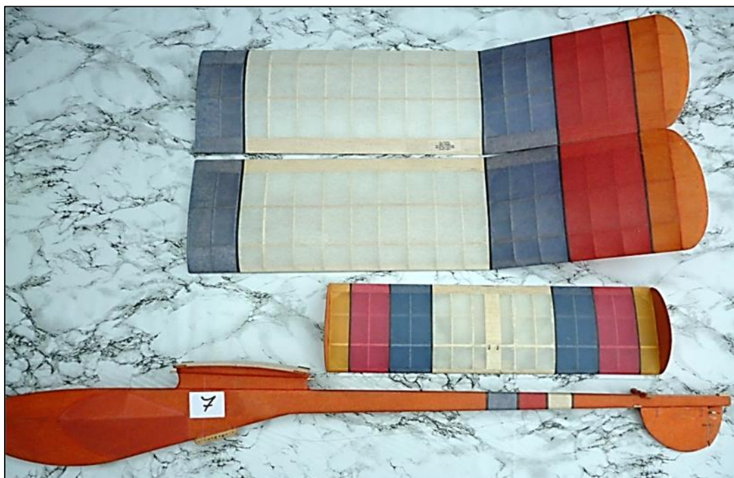
No 7: Wing Span 146cm; Chord 18cm; Fuselage length 108cm
