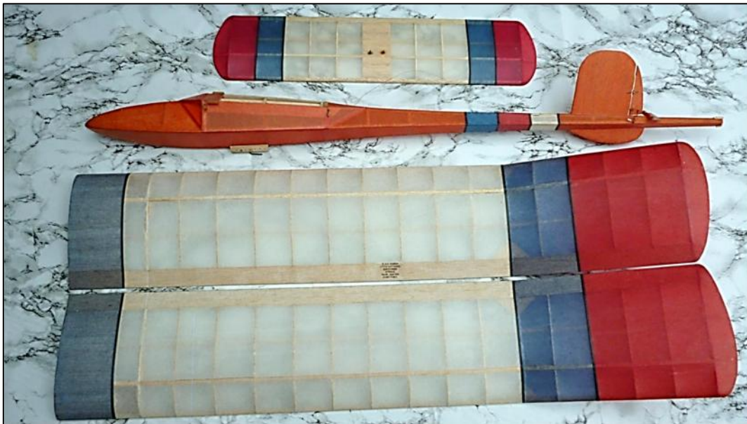
No 9: Wing Span 172 cm; Chord 16cm; Fuselage length 92cm – AH20?
