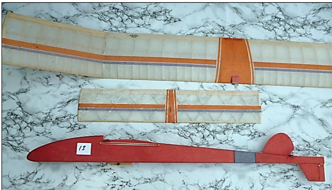
No 13: Wing Span 149cm; Chord 17cm; Fuselage length 94cm
