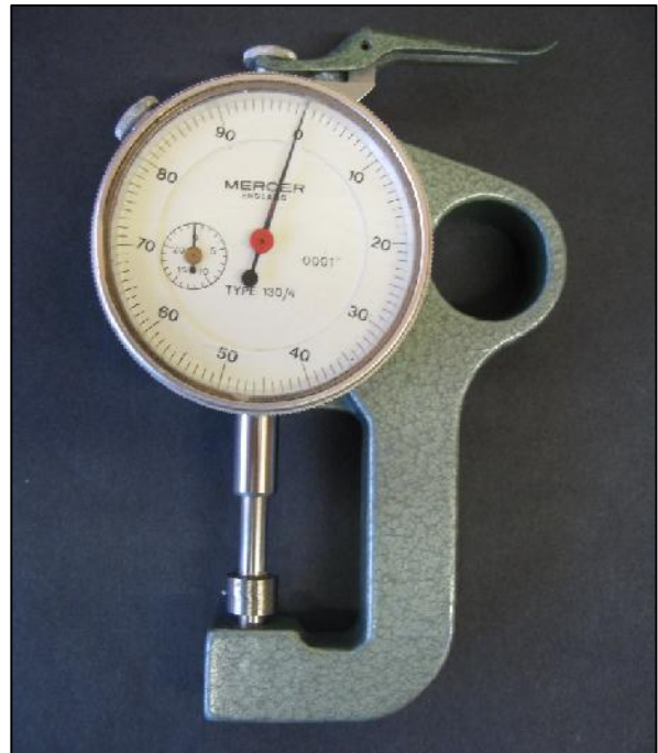
Fig 5. Dial thickness gauge for measuring rubber strip width.
