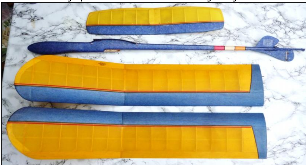
"A": Wing Span 193 cm; Chord 16 cm; Fuselage Length 125 cm
