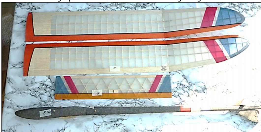
"C": Wing Span 93 cm; Chord 16 cm; Fuselage Length 107 cm
