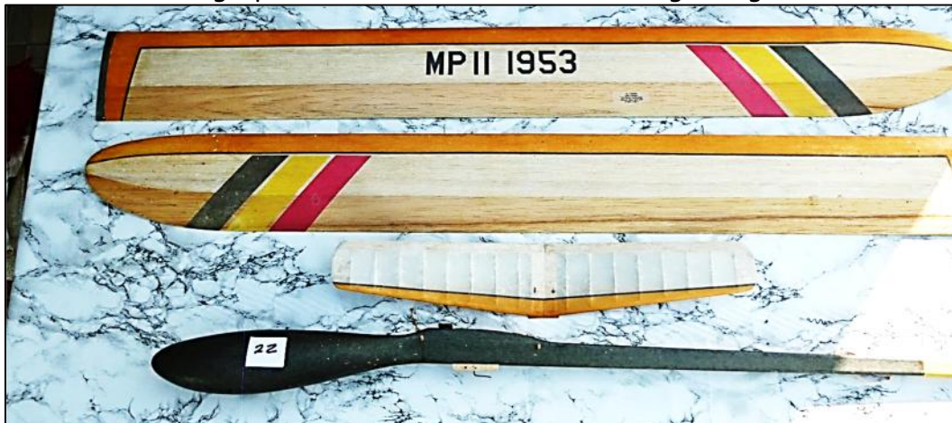
No 22: Wing Span 236 cm; Chord 13.5cm; Fuselage Length 145 cm
