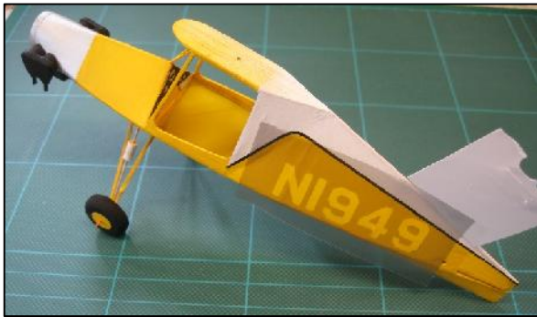
Fig. 5. Registration letters cut from Ultra Mask film and attached to fuselage side.
