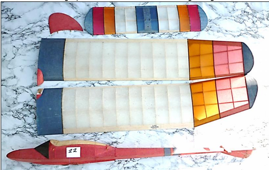
No 23: Wing Span 160 cm; Chord 18 cm; Fuselage Length 92 cm
