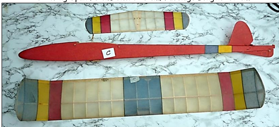
"C": Wing Span 93 cm; Chord 16 cm; Fuselage Length 107 cm
