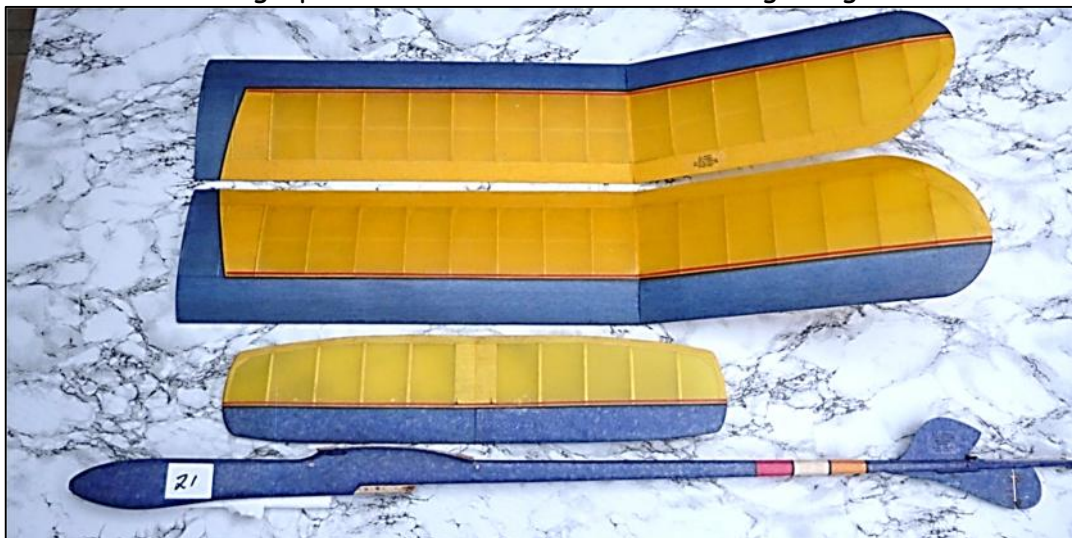
No 21: Wing Span 176 cm; Chord 16.5 cm; Fuselage length 90 cm
