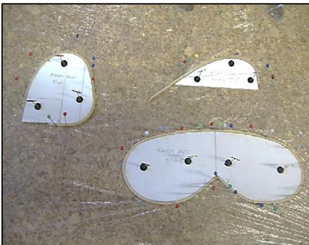
Laminated tail surface outlines and wing tip
