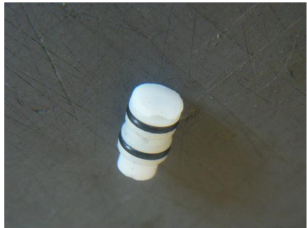
Valve cartridge assembly with cap in place (GM photo).
