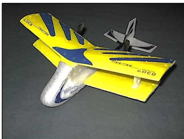
Silverlit X-Twin Bi-Wing, 220 mm wingspan, 18 g weight
