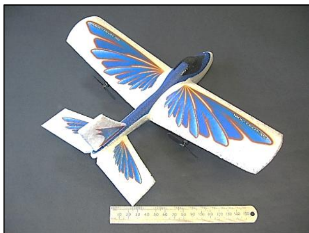
Silverlit X-Twin Sports Flyer, with propellers behind the wing trailing edges
