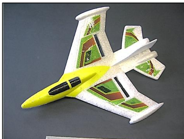
X-Twin Jet (propellers in wing slots)
