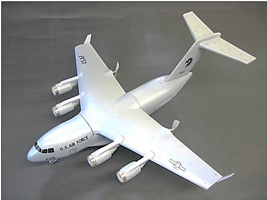
390mm wingspan, six engine C-17 transport – four dummies and two pushers at the wing trailing edge.
