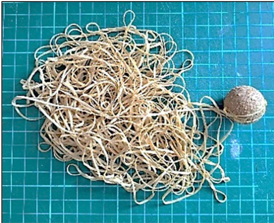
Stage 8 Completely unwound revealing core
