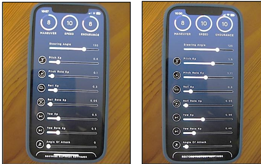
POWERUP 4.0 App settings screen for Invader paper glider (left) and Tornado Updraft 12 balsa plane (right).
