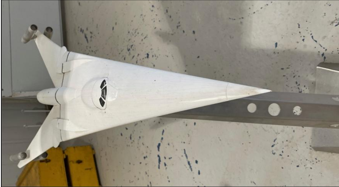
A model of the Vickers Swallow, submitted as a proposal by Vickers as one of the competitors to the TSR2 bid. Designed by Barnes Wallis & years ahead of its time in concept.
