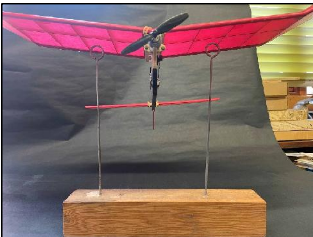
Checking the cg position of the Micro-Starduster. Note the coil of cored solder around the motor as nose weight.
