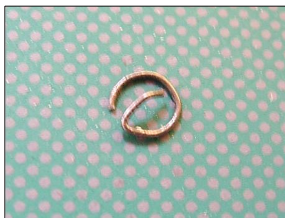
0.020" dia. wire ball retainer. The od is around 6mm.
