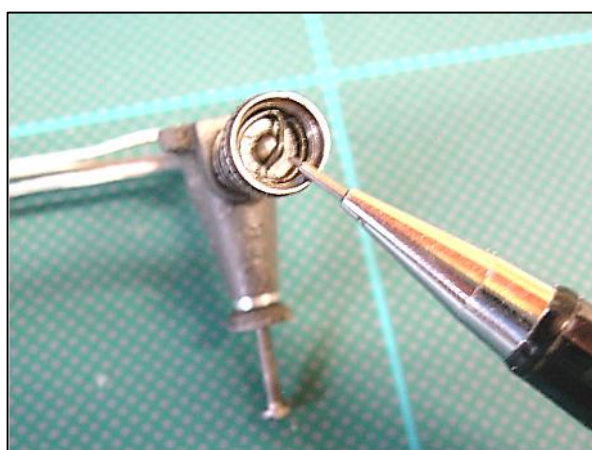
Ball valve and retainer in cylinder head of Junior .005 motor.
