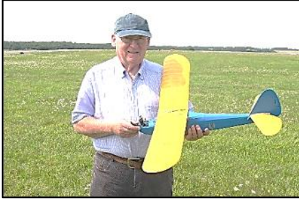
Trevor Jones with his 40" wingspan Miss Arpiem, powered by a Mills .75 This is a reduced size version of the design by Steve Kowalik. (right photo by Peter Carter)
