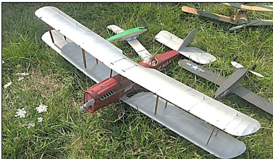
Mike Smith's splendid F/F Scale Nats winning 51" wingspan DH4 Mailplane, powered by a Mills 1.3.
