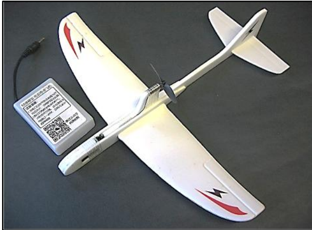
'Airy' foam plastic supercapacitor powered ARTF aircraft.
