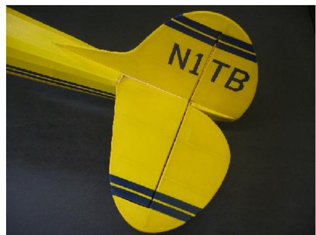
Fig 4. Finished tail surfaces, also showing frame for fin/stabiliser fairing
