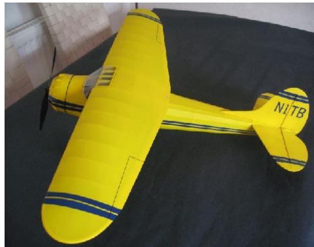
Completed Cessna 195, modified for three channel RC based on Earl Stahl plans, August 2021. Weight 221g.
