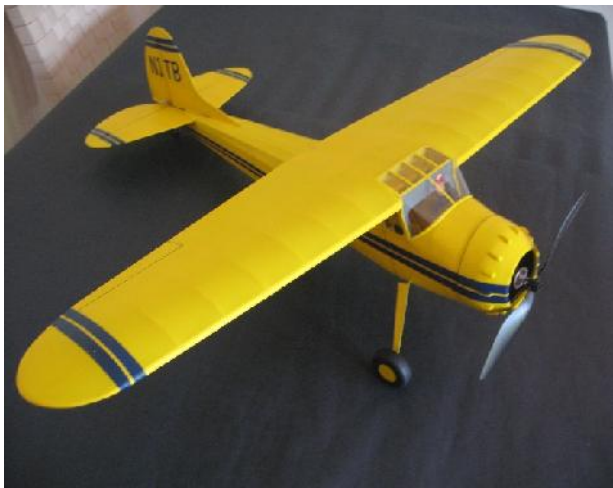
Completed Cessna 195, modified for three channel RC based on Earl Stahl plans, August 2021. Weight 221g.
