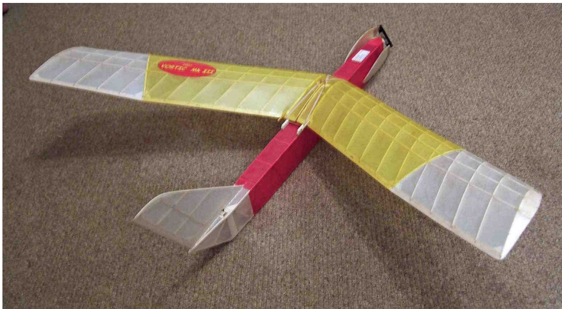
Vortic III, less elevons, but otherwise ready to go (note the 'reverse' angle ribs at the trailing edge break)
