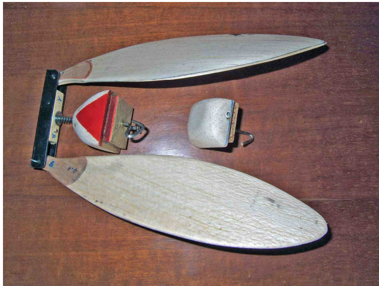
I went for my favourite 2 blade folder with laminated blades. Dummy noseblock for lower motor on right
