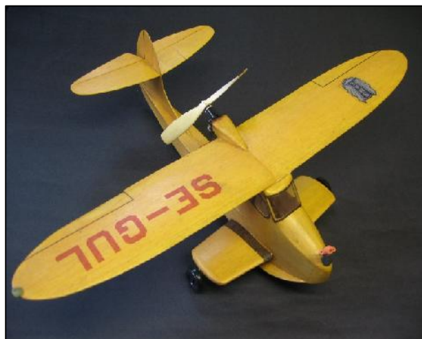
Two views of the Tadpole, powered by a Telco CO2 motor (60mm3). Weight 48g
