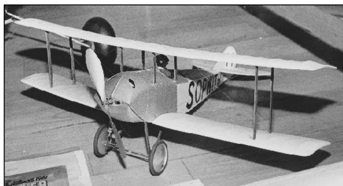
5/72 scale Sopwith Tabloid powered by Brown MJ 140 CO2 motor at Model Engineer Exhibition in 1983. Weight 68g.
