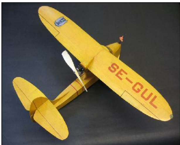
Two views of the Tadpole, powered by a Telco CO2 motor (60mm3). Weight 48g
