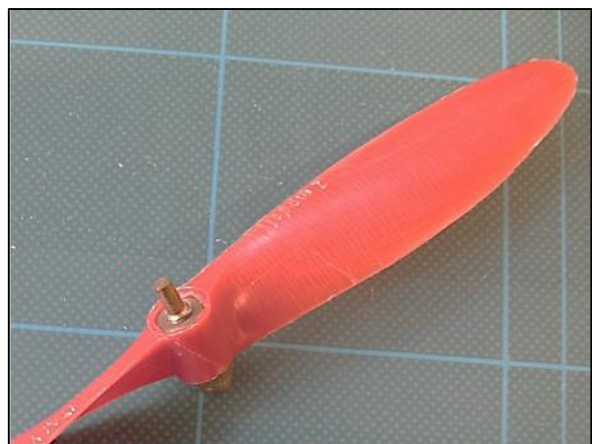
Z Model propeller –stress crack lines can be seen on the upper blade
