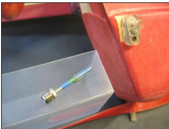
Transparent filler valve and nozzle and improvised filler adaptor.
